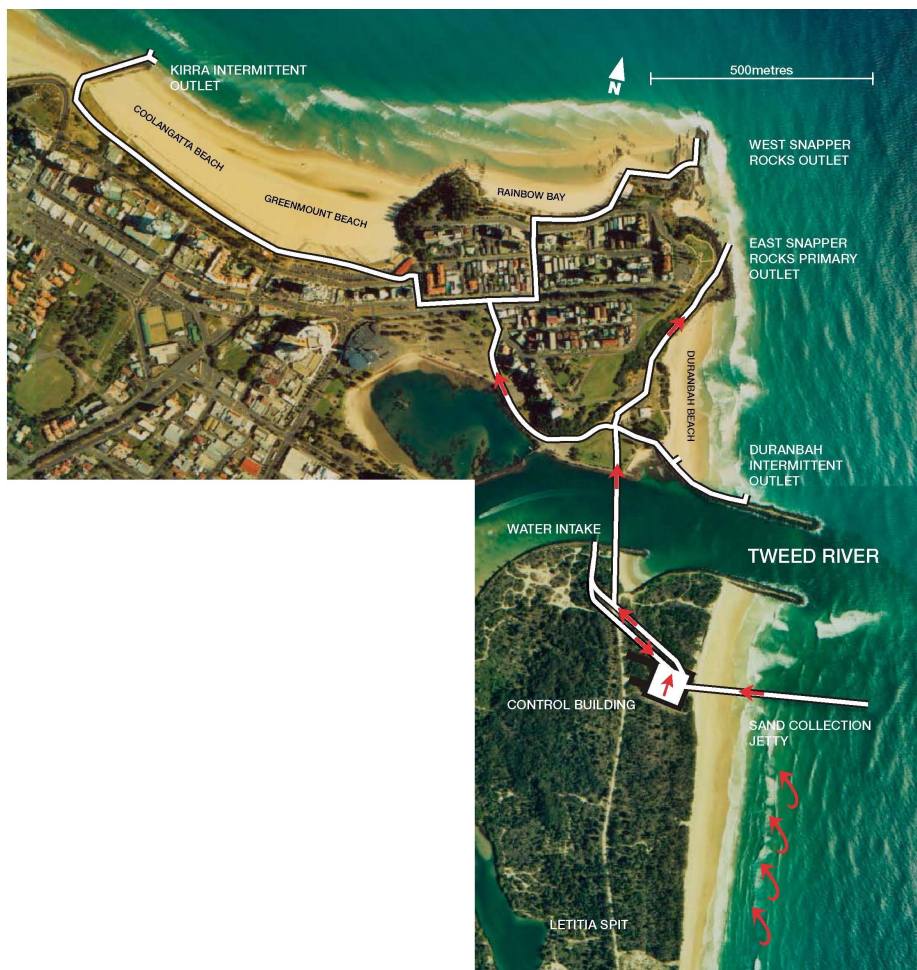
Figure 3 Jetty-based sand bypassing system components
